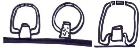
Figure 2 Hole is recessed so there is space for the stopper end above the table plane.
