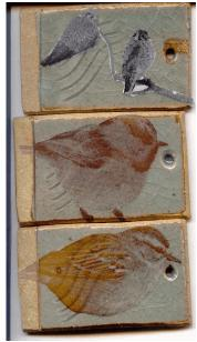
Top: unfired decal applied to cone 10 celadon Middle: fired to cone 02 Bottom: fired to cone 2
