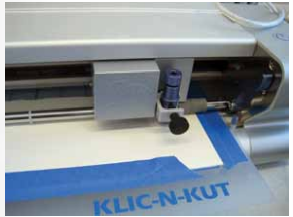
The completed template files are then sent to the die cutter and cut from 300-pound watercolor paper.
