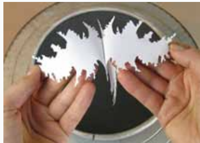
Separating the double-thick friskets before use. The die cutter cuts better with slightly heavier materials so two sheets are laminated for cutting.
